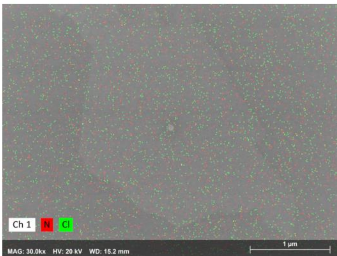
Figure S9. EDS image after applying R6G on the coated MXene substrate.
